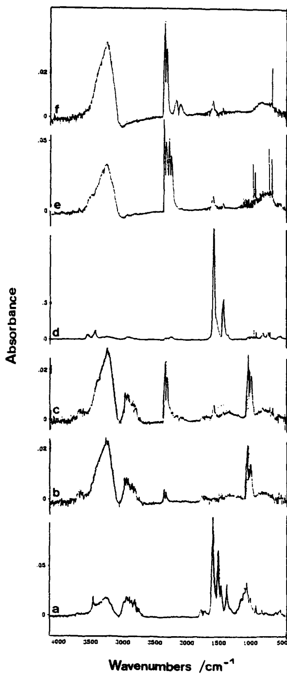
Fig. 3. FTIR spectra performed at: a, 175°C; b, 265°C; c, 395°C; d, 410°C; e, 525°C; f, 660°C.
